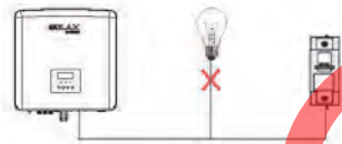
Figure: Wrong connection of load and inverter
